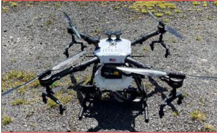
AG-110, 2.6 gal tank, 20 ft swath, 15 ac/hr
